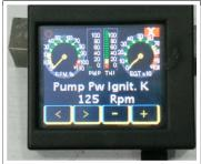
Next is the setting for minimum pump speed during the start.
