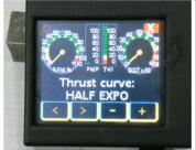
THRUST CURVE. You now get to the setting for thrust curve (as indicated in the chart).
