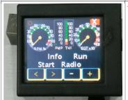
There are no more functions to adjust in this branch so exit by pressing > until you return to the opening screen.
