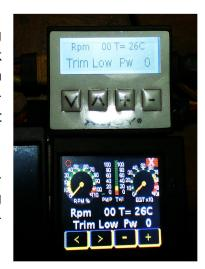
Both displays include dedicated screens for engine operation, radio checking, last shutdown cause and other special turbine operations.
