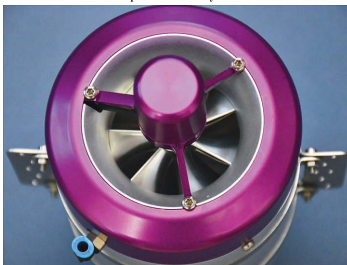
Close up view showing very nice machining on the compressor and the single fuel connector.
