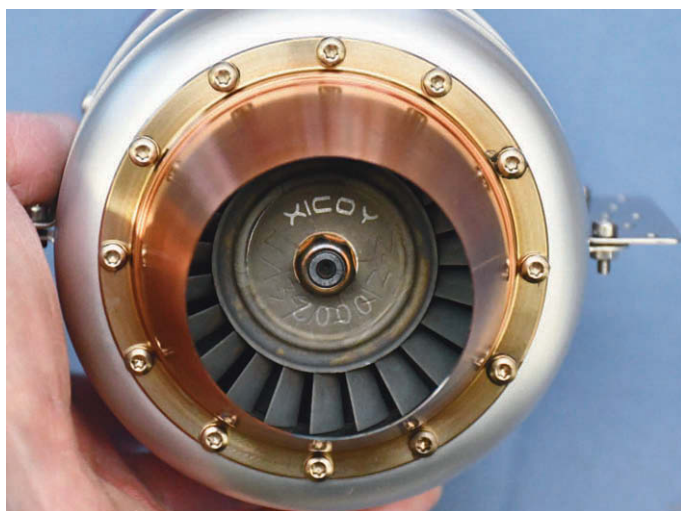
View of the turbine wheel showing the neat casting of the blades, these requiring minimal balancing work.
